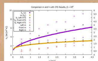
Figure 7.- Results for the  $m$  parameter and  $h$  coefficient at a case of a fluid flow of  $v = 1$  m/s and an attack angle of  $\beta = 45^\circ$ .
