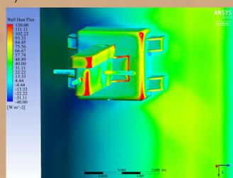
Figure 6.- Convective heat flux distribution over the HABIT-Pole structural model.
