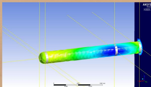
Figure 1.- Air Temperature Sensor 3D model for CFD studies.
