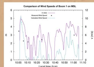
Figure 5.- Model approximation to wind speed measurements of MSL mission sol 547.
