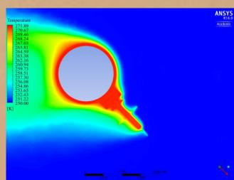
Figure 4.- Horizontal section for the thermal wake at a case of a fluid flow of  $v = 1$  m/s at  $T_f = 250$  K.
